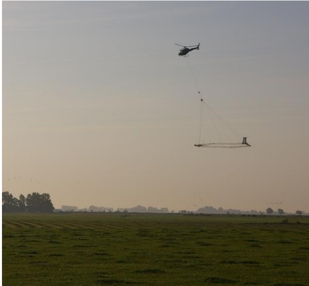
Figure 2: Helicopter with measurement frame
